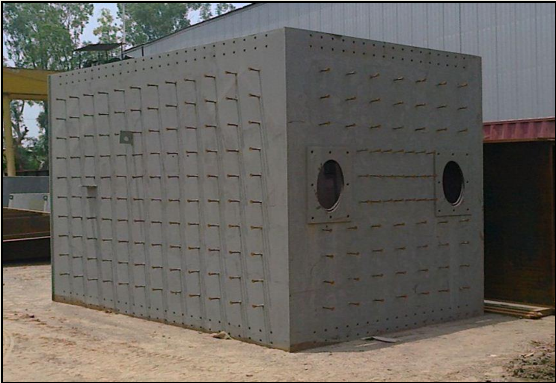
Fabricated Box Section for Steel Pylon
