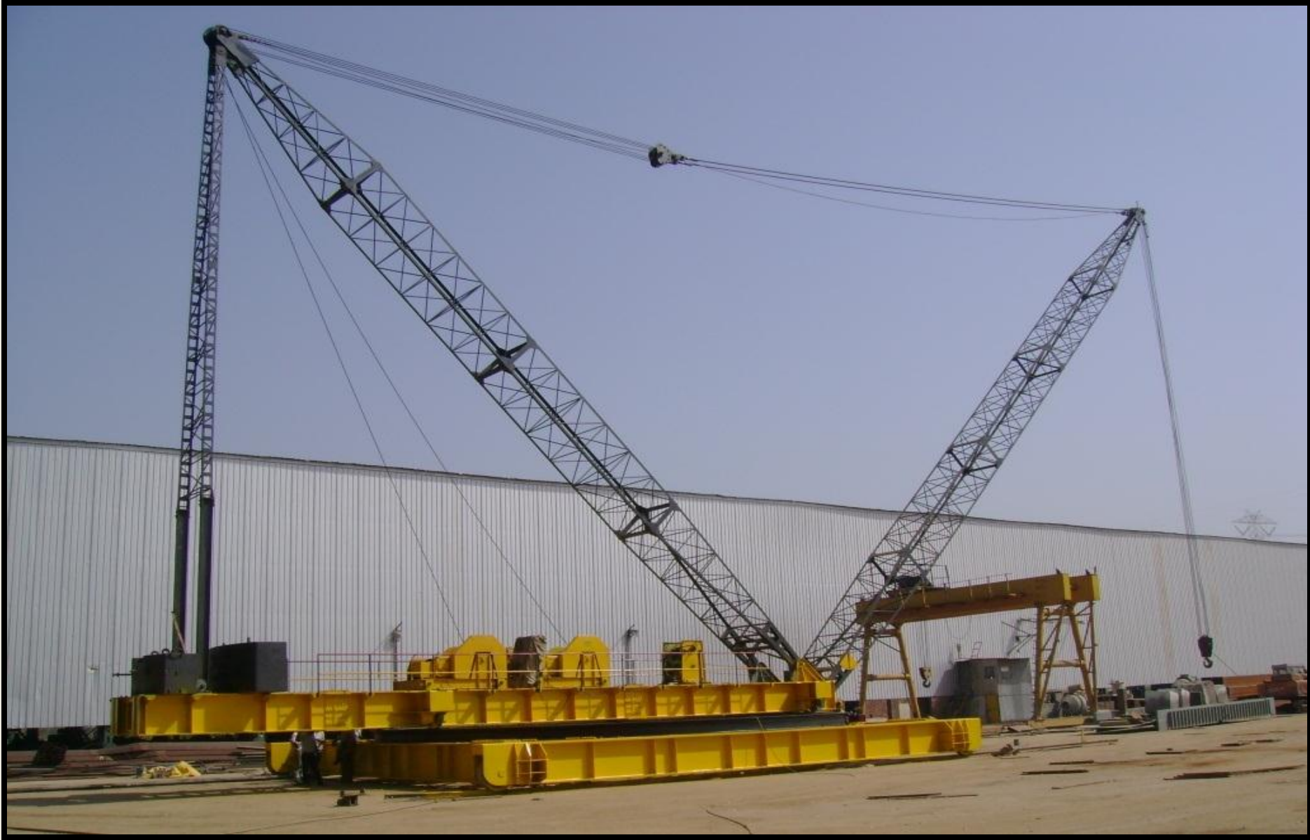
Fabricated Erection Crane of Capacity: 20MT
