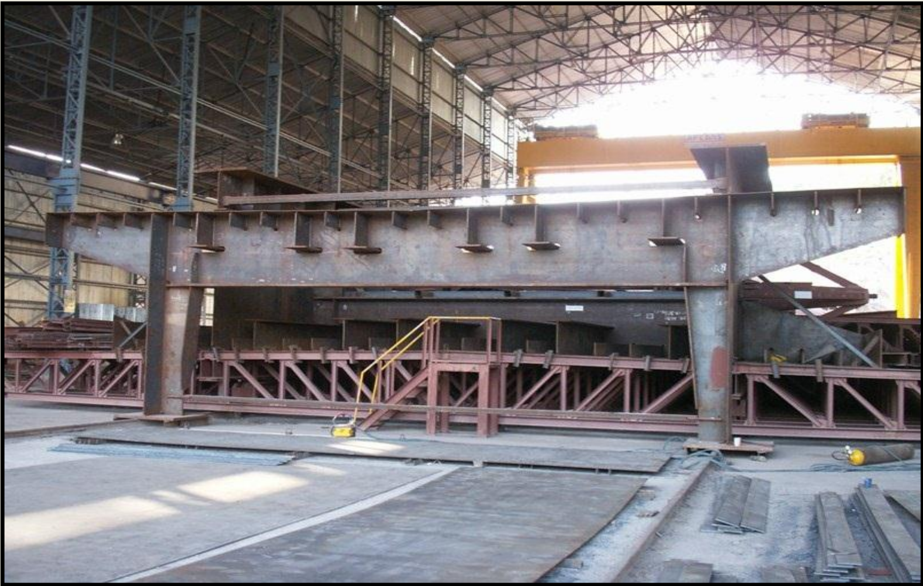
Built up Steel Deck (for Chenab Bridge) inside a Workshop Bay
