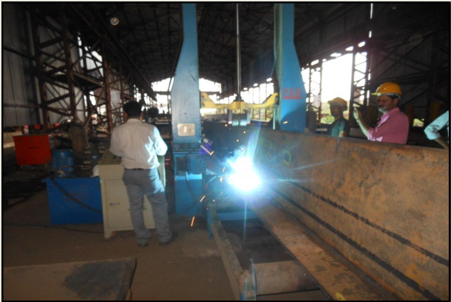
Fit-up of Longitudinal Girder
